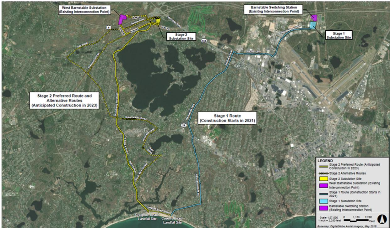
The on-shore cabling routes for Stage I and Stage II. The Town will be installing public sewer lines along the same routes saving millions of dollars in construction cost and avoiding multiple construction disruptions by performing the work simultaneously.
